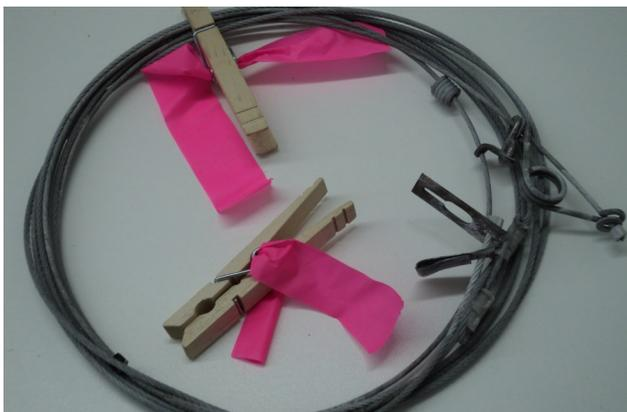
Figure 17. Colored survey flagging threaded through the center of hinged clothespins works well for keeping cable devices organized and identifying set locations. Attach one to each coiled cable device when storing the cable; remove it and attach it to nearby vegetation or another structure to identify the set location once the cable device is set; and recover when the cable device is removed.
