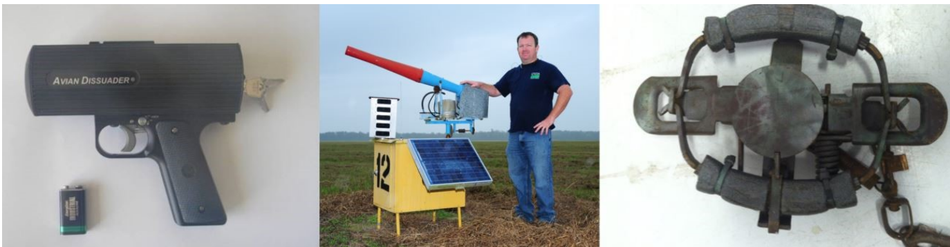
Figure 4. Frightening devices used to disperse ravens include lasers ( left ) and propane cannons. Modified soft-catch traps are also used to live trap the birds ( far right ).
