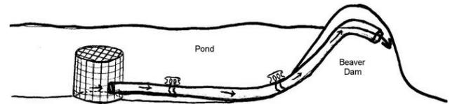
Figure 6. An example of a flexible pipe with a round fence used to control the water level at a dam.
