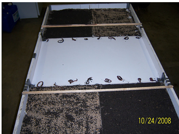
Figure 1. We conducted experiments on the National Aeronautics and Space Administration's Plum Brook Station, Ohio, USA, during 2007–2011 to identify products that could be used to repel or suppress nonnative earthworms on airports or other managed sites. Simulated runway experimental apparatus showing 1 of 2 tables with a central area from which earthworms would move into soil quadrants. One table contained 2 quadrants of treated and 2 quadrants of control soils, while the second table served as a control table.
