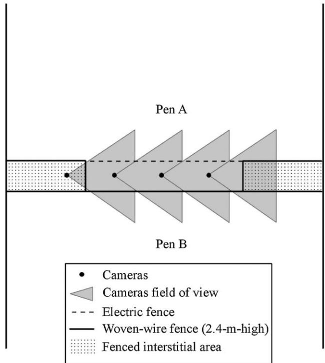
**Figure 1.** Layout (not drawn to scale) of test-fence area and video surveillance system examining efficacy of an electric fence to reduce contact along fence-lines by farmed elk in north-central Colorado, USA. Cameras were orientated in the same direction to yield continuous coverage of the test-fence area. We monitored the test-fence area between August 2006 and October 2007.
