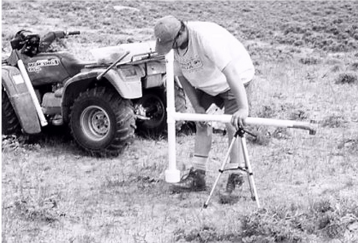
Figure 3. Optical Sighting Device. The device is set as close as possible to the selected coordinates. Cross-hairs on the objective lens in the sighting tube pinpoint the spot for each reading as the apparatus is stopped at 30 degree intervals around the circumference of a one meter circle.
