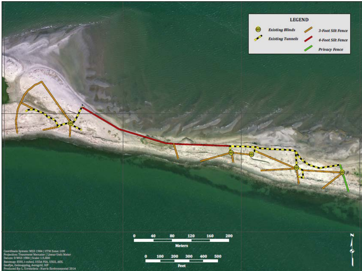
FIGURE 2-5. Example of additional silt fence and existing structures that would be used to delineate lethal removal areas, and reduce disturbance to non-target birds on the DCCO breeding colony on East Sand Island.
