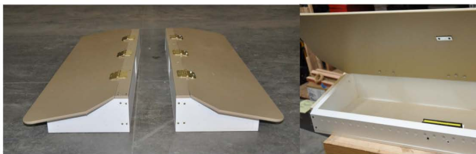
(upper left) -Complete feeding device. Note the handles also serve as 'stoppers' to prevent the lids from remaining open once feeding ceases. (upper right) - Frontal view of the device with the lid propped open. (lower left) - Two halves of the feeding device. (lower right) - Example of the magnetic locking mechanism.
