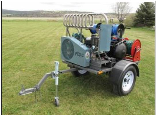
Figure 2. The PERC<sup>®</sup> machine used to fumigate burrowing rodents.
