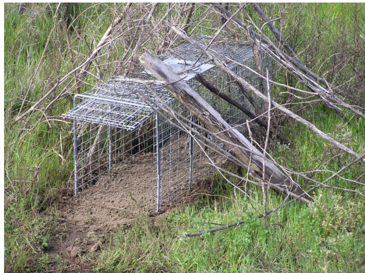
Figure 1. Standard box trap, often called a cage trap, set for a raccoon. The pan is in the rear and attached to the door by a metal rod. When the door closes, a hinge opens another flap that does not allow it to be opened from the inside.
