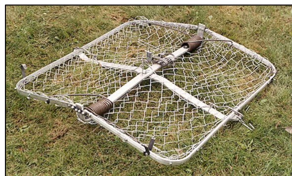
Figure 6. Bailey trap, a purse trap, used primarily for trapping beaver. This purse trap has a size of 39" x 21" x ~12" and weighs about 30 pounds.
