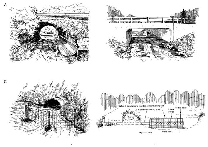
FIGURE 15.3. Examples of water control structures used to manage beaver (Castor canadensis) impacts. Source: Adapted in part from Jensen et al. (1999).
