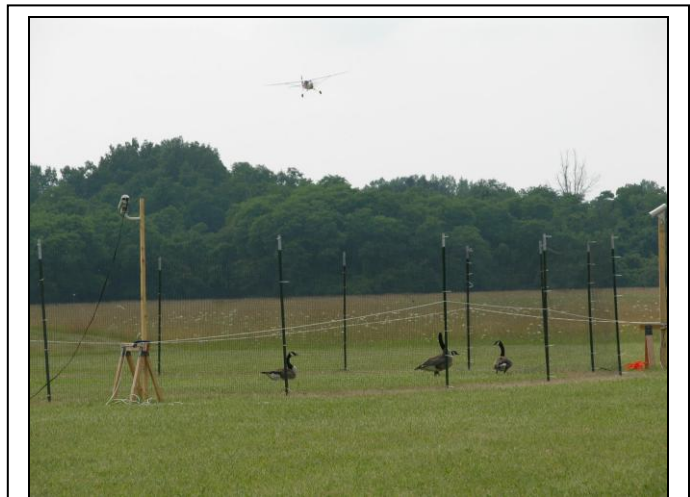
A remotely-controlled aircraft approaches a group of captive Canada geese in an experiment in Ohio in 2010 to determine if aircraft lighting systems can be modified to enhance bird detection and avoidance of aircraft (Blackwell et al. 2012). Photo, G. Keirn, USDA.
