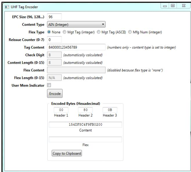
If you have the encoding for a tag and would like to reverse the process above, then you can use the Decode option in the sample app selector.
