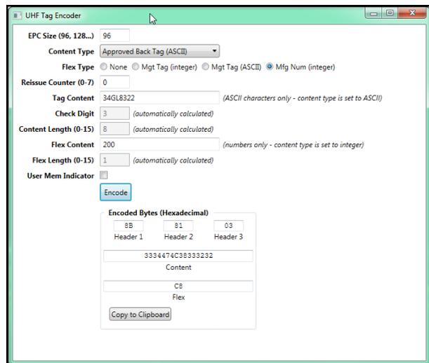
Click on Encode and the Encoded Bytes in Hexadecimal fill the Header, Content and Flex fields. In this example the result is 8B81033334474C38333232C8.
