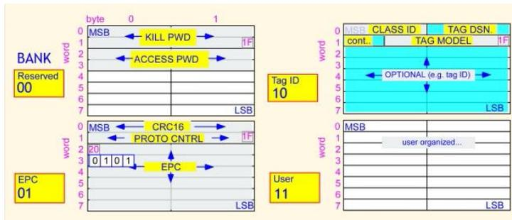
The interim TDS described in this document divides the Class-1 Gen 2 EPC memory into three general sections (not including the CRC and PC): **Header**, which occupies the first three bytes, the **Content** section that holds the actual device identification and a **Flex** section that may or may not be used to store additional information.
