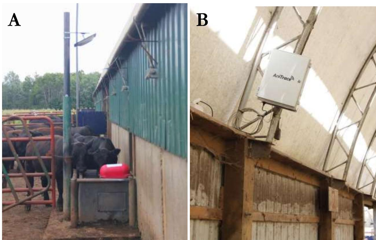
**Figure 3.** AniTrace system installed at MCA/MSU Bull Evaluation Program Station, Crystal, MI. Antennas were mounted directly above outdoor automatic waterers (panel A). Reader boxes were mounted inside adjacent hoop barn (panel B). Remote Internet connectivity was extended from the station residence wirelessly by an Ubiquiti bridge, Ubiquiti receiver, and ASUS wireless router.
