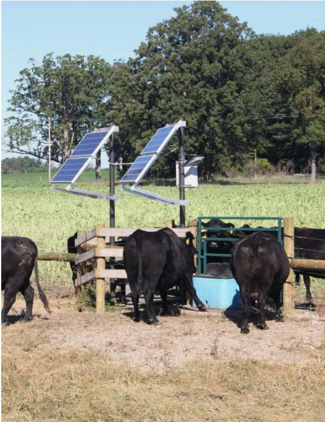
**Figure 5.** UHF RFID read point (AniMonitor, division of Hana Micron America; Milpitas, CA) that is solar powered at the MSU Beef Cow/Calf Teaching and Research Center. Antenna is located directly above an automatic waterer which is split between two pastures.
