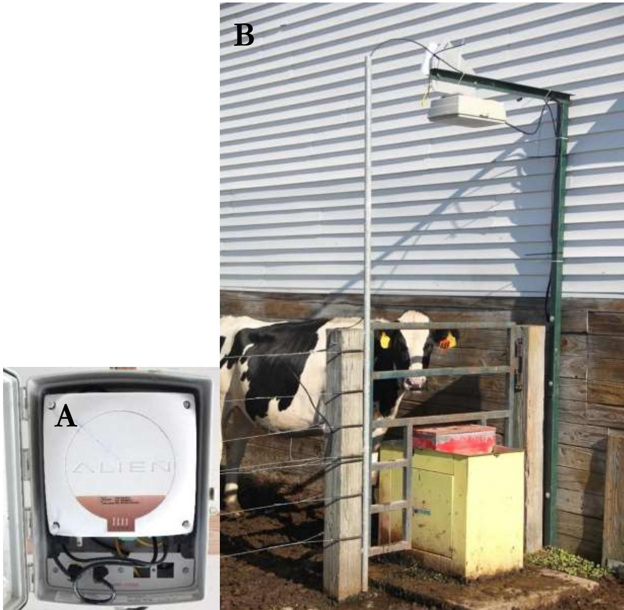
**Figure 1.** A weather-resistant enclosed ALR-9650 Gen 2 RFID reader (Alien Technology San Jose, CA; panel A) located directly above an automatic waterer in an outdoor beef feedlot application (panel B). Remote Internet connectivity was provided by an Arymesh network (Ayrstone Productivity, LLC, North Oaks, MN).
