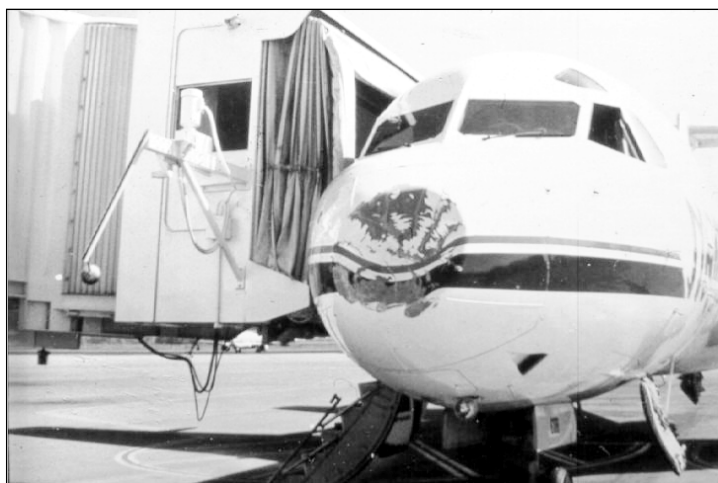
Figure 15. Just prior to landing at 50 feet above ground level, this aircraft struck a Red-tailed Hawk damaging the radome which disabled the navigation system. The passengers and crew experienced significant vibrations during landing. The pilot landed the aircraft safely, but emergency vehicles responded to ensure that mishaps did not occur.
