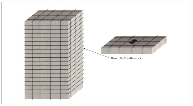
Figure 3-7-3 Fruit Stack with Middle Row Temperature Probe Placement
