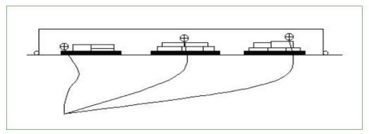
Figure 2-4-3 Example of the Position of Gas Sampling Tubes (Side View)
