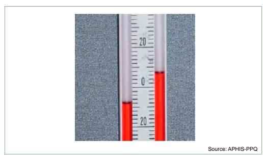
Figure 8-1-8 Example of U Tube Manometer
