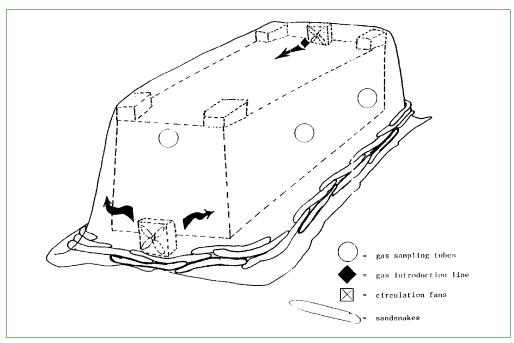
Figure 2-4-4 Typical Break Bulk Arrangement with Fans, Leads, Introduction Line, Padding, and Sand Snakes
