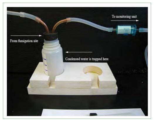
Figure 8-1-9 Example of a Water Trap
