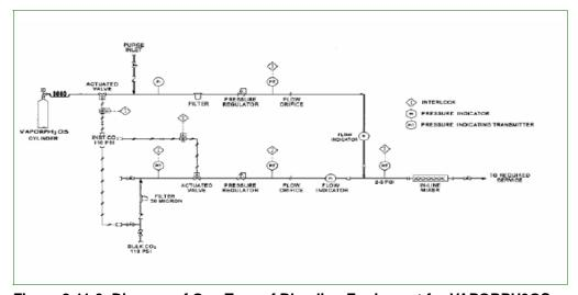
Figure 2-11-3 Diagram of One Type of Blending Equipment for VAPORPH3OS
