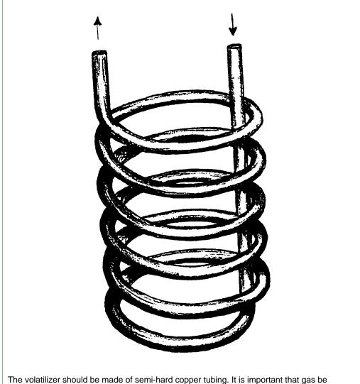
The volatilizer should be made of semi-hard copper tubing. It is important that gas be introduced and discharged as shown by arrows. If applied in reverse order, it may move so rapidly that some liquid will pass into the chamber.
