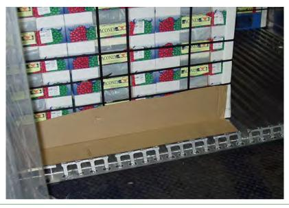
Figure 3-7-5 Proper Placement of Cardboard Between the Last Pallet Row of Fruit and the Back Doors of the Container
