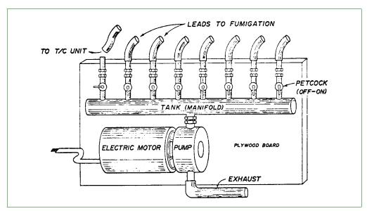
Figure 8-1-6 Auxiliary Pump
