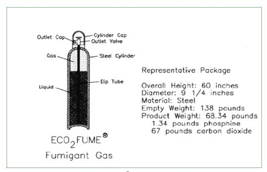
Figure 2-11-1 Diagram of ECO<sub>2</sub>FUME<sup>®</sup> Gas Cylinder
