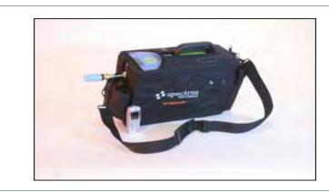
Figure 8-1-3 Spectros Methyl Bromide Monitor
