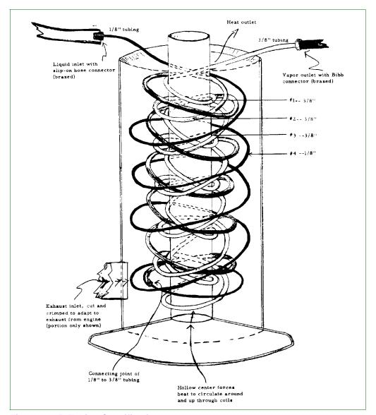
Figure 8-1-5 Tubing Specifications
