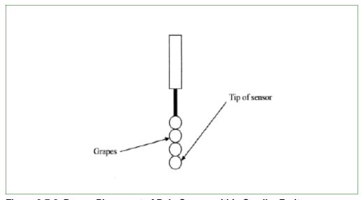
Figure 3-7-2 Proper Placement of Pulp Sensor within Smaller Fruit
