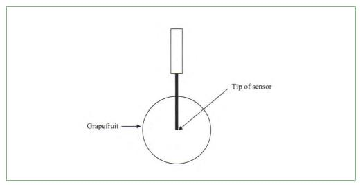
Figure 3-7-1 Proper Placement of Pulp Sensor within Larger Fruit
