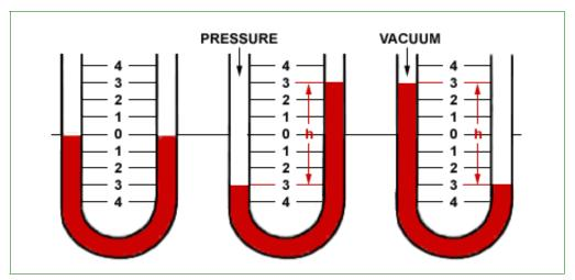
Figure 8-1-7 Example of Pressure Measurement in an Open-arm Manometer
