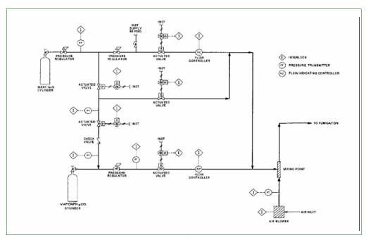
Figure 2-11-4 Diagram of VAPORPH3OS® and Forced Air Blending Equipment
