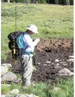
digital images may be used to trace the field perimeter and calculate the area using GIS software.
