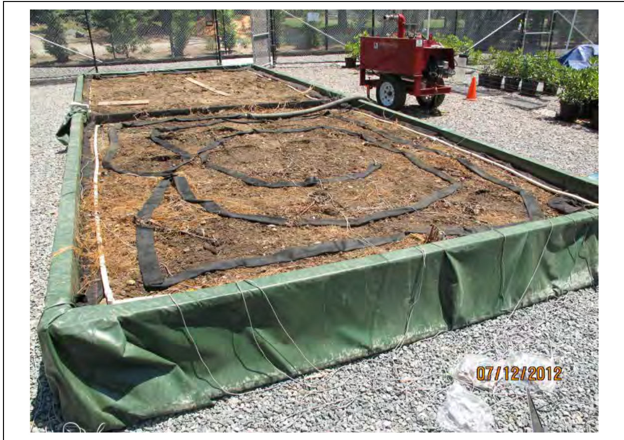
Figure 14-1 Steam Sock in Place on Soil Surface
