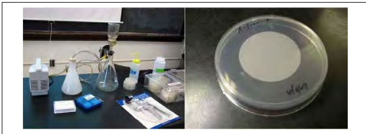
Figure 12-6 Vacuum Apparatus for Water Filtration and Filter Plated onto PARPH-V8 Plate 2
