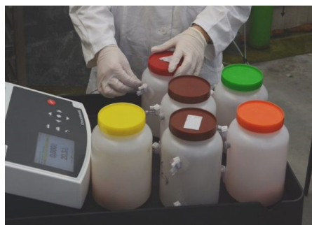
Figure 2. Measurements of O 2 and CO 2 levels were taken from containers holding infested fruits.
