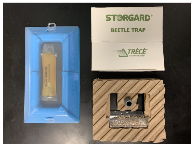
Figure 1. Traps deployed at distillers' dried grains with solubles production facilities included an Insect Limited™ floor trap with pheromone gel (left) and a Storgard APHIS KIT-KB wall trap with wheat germ and pheromone lure (right).
