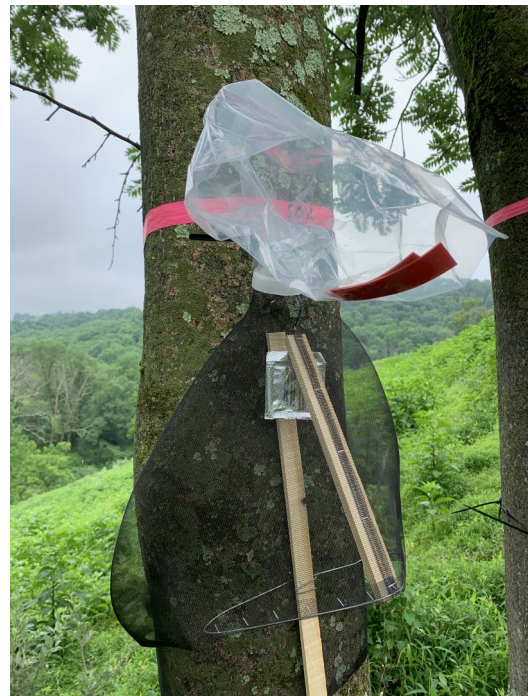
Figure 2. SLF circle trunk trap design with a plastic gusseted bag, developed in 2019.
