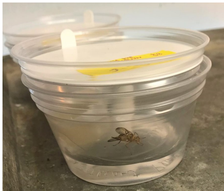
Figure 1. Diet arenas consisted of a lower cup serving as a water reservoir and an upper cup with a hole in the bottom, placed over the water. A dental wick protruded from the reservoir into the upper cup to serve as a water source. Diets were offered in polyethylene dishes in the upper cups.
