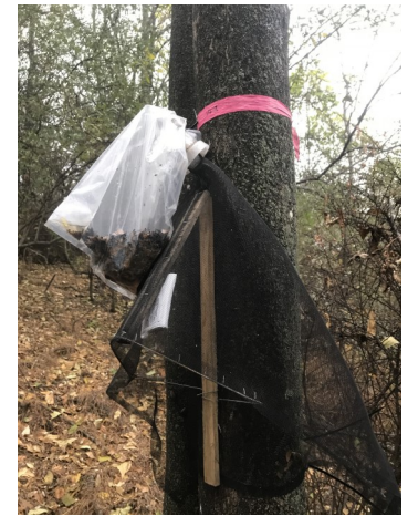
Figure 6. Bag collection device during adult flight during a periodic check. Three weeks had passed since the trap had last been checked.
