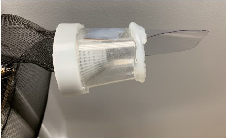
Figure 3. Depicted is the original pecan weevil collection cup modified for the bag collection device. The end of the cup is removed and acetate sheeting is attached to the top of the cup. A line of hot glue is placed around the edge of the cup to provide a synch point for the cable tie.
