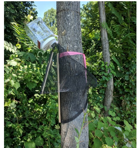
Figure 3. A circle trunk (modified pecan weevil trap) placed on an Ailanthus host. The collection jar size has been increased and the entrance has been widened to accommodate large SLF.
