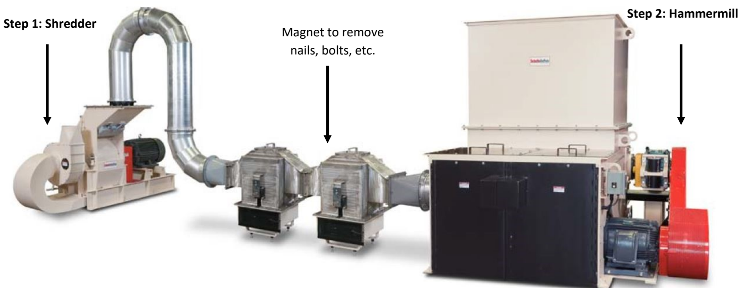
Figure 1. Equipment tested for the destruction of abandoned dunnage and pallets at the port of Houston, manufactured by Schutte-Buffero.
