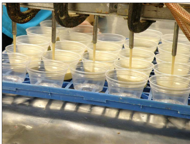
Figure 1. Gypsy moth artificial medium being dispensed into rearing containers via an in-house designed manifold.
