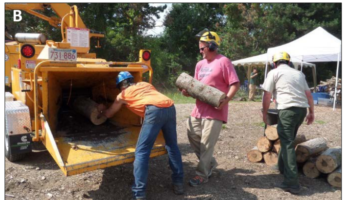
Figure 1. A) Artificially seeding logs with surrogate larvae. B) Loading drum/disc chipper with ALB infested maple logs.
