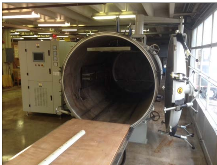
Figure 1. A custom-built radio-frequency oven, to be used in developing the phytosanitary treatment for wood packaging material.
