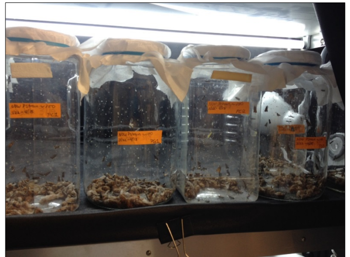
Figure 2. Emerged adults from infestation density studies. The study was combined with a comparison of glass and plastic jars.
