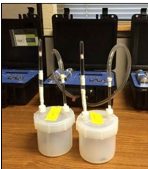
Figure 3. Portable volatile collection system used to collect headspace volatiles from adult VLB.
