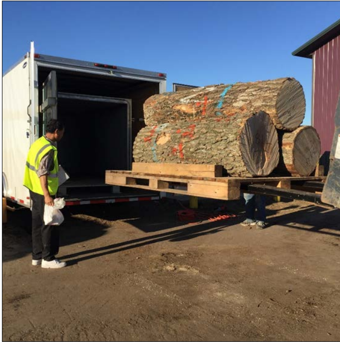
Figure 3. The portable vacuum steam chamber being loaded with oak logs.
