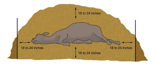
Figure 2. Dimensions of carcass in windrow (Illustration by Josh Payne)
