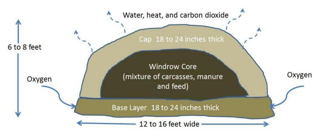
Figure 1. Cross section of compost windrow (Illustration by Gary Flory)
