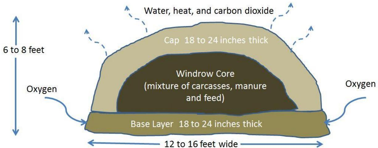
Figure 1. Cross section of compost windrow (Illustration by Gary Flory)
