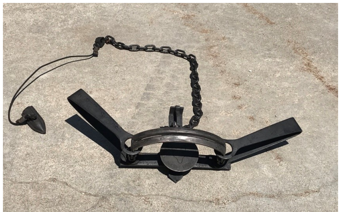
Figure 13. Foothold trap equipped with a “bullet” anchor which is driven into the ground. When the chain is pulled, the anchor pivots, anchoring the trap in place.
