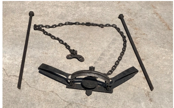
Figure 12. Foothold trap configured with two stakes for anchoring the trap in place.
