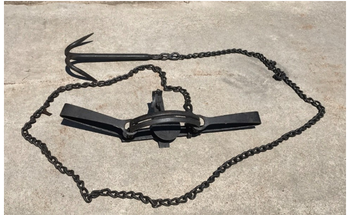
Figure 11. Foothold trap configured with chain and 2-pronged drag-hook.
