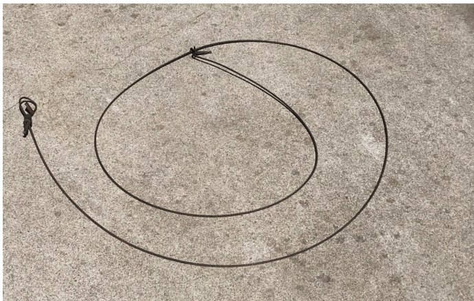
Figure 15. Cable restraint devices are made of varying lengths and sizes of wire or cable looped through a locking device that allows the loop to tighten.
