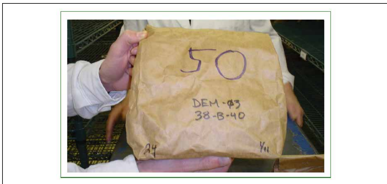
Figure 4-3 Sample Beaker Number (50), Collection Number (DEM-03), Field Name (38-B-40), Sample Bag Number (24), and Collection Date (1/11)
