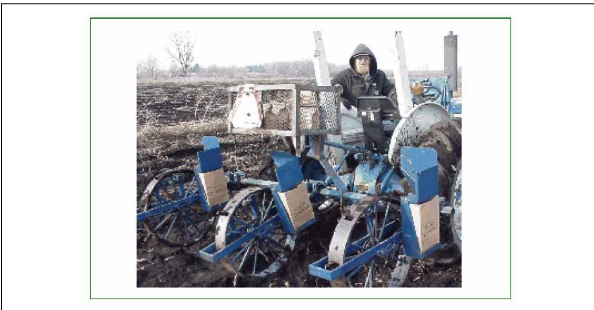
Figure 3-5 Three-Wheeled Mechanical Sampler
