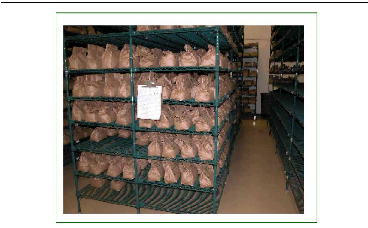
Figure 4-2 Soil Samples Drying in the Rack Room
