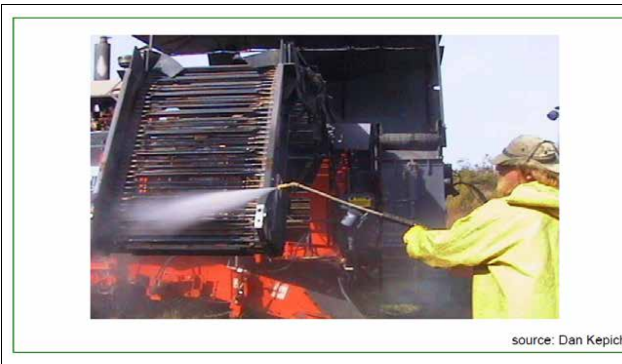
Figure 7-2 Pressure Washing with a Single-Orifice Nozzle
