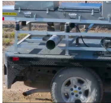
Flies are dispersed directly into the air from a truck with a sterile fly chamber on the back. They may also be released from ground release chambers—covered crates that allow the pupae to hatch and fly into the open air.
