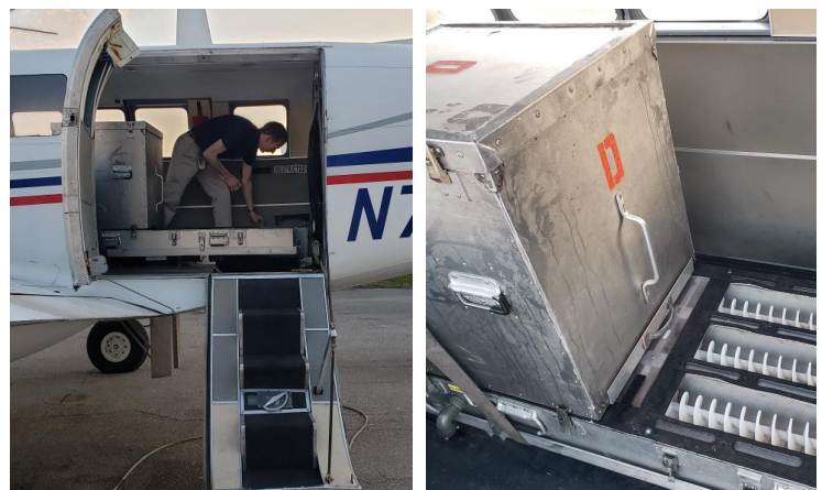
Specialized sterile insect dispersal aircraft being loaded with sterile NWS flies for dispersal. The chamber holds the flies and connects to the auger in the plane and moves the flies directly outside once the plane is in the correct location.
