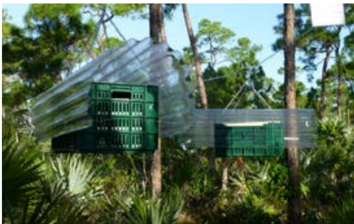
Sterile insect ground release chambers | USDA photo, D. Bonilla
