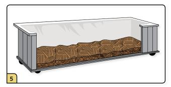
Rake one foot of absorbent material on the container floor with a heavier concentration near the rear door. Close container and adjust plastic and absorbent material as needed.
