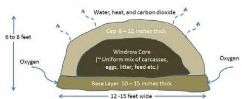
Figure 1. Cross Section of Compost Windrow
