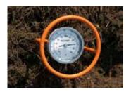
The purpose of windrow composting of HPAI related poultry carcass mortality is inactivation of avian influenza virus. Compost pile temperature measurements are a critical indicator of effectiveness of the compost process for virus inactivation. Temperature monitoring is performed by a compost subject matter expert (SME), regulatory monitoring staff, contractors, or farm personnel. Accurately monitoring and recording daily
