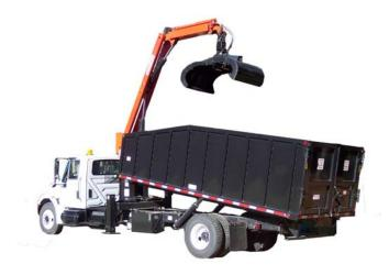
Figure 2: Grapple truck with dump trailer.
