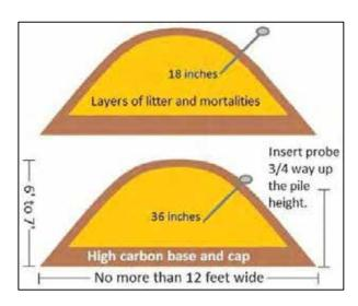
➤ Leave the thermometer at each depth and point for at least 60 seconds.
