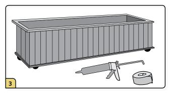
Inspect and line the containers. Seal any holes or spaces with duct tape, plastic liner, caulk, or silicone. Return containers that you cannot seal.
