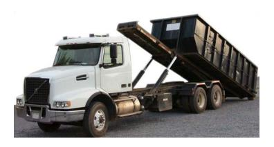
Figure 5: Example of a roll-off truck trailer.
