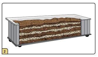
Load carcasses evenly. Alternate one foot of absorbent material with each layer ending with absorbent material.
