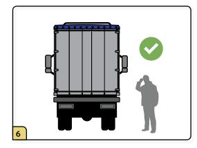
Disinfect and inspect vehicle before departure. Verify the load is not too large, and there are no leaks, cuts, or holes. If the load is dripping, the contents must be transferred to a correctly lined container.
