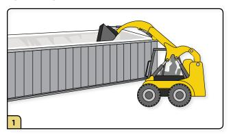
Load container with carcasses using a skid steer loader and/ or front-end loader. Ensure carcasses are not placed on the ground while moving from the staging area to the container.
