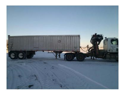
Figure 1: Standard Rendering Truck with Grapple System
