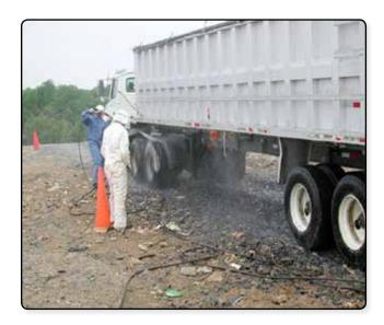
Following offloading, the trailers will be washed per incident-specific protocols and will be cleaned at a commercial truck wash prior to returning to service.
