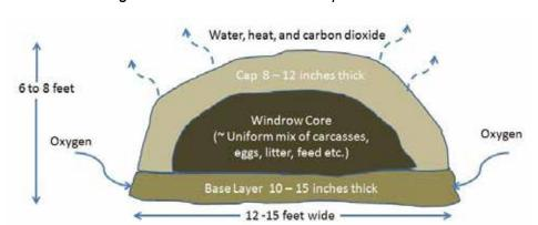
Figure 1. Cross Section of Compost Windrow
