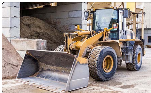
Pay loader used for clearing the base
