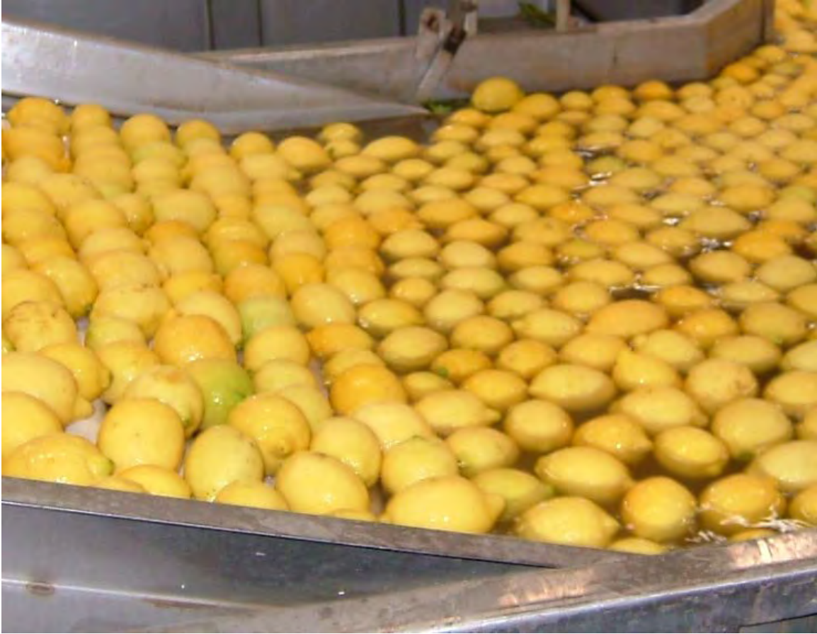
Packing line, floating through sodium hypochlorite and then up ramp to be dried and brushed, Argenti Pack House, August 7, 2007
