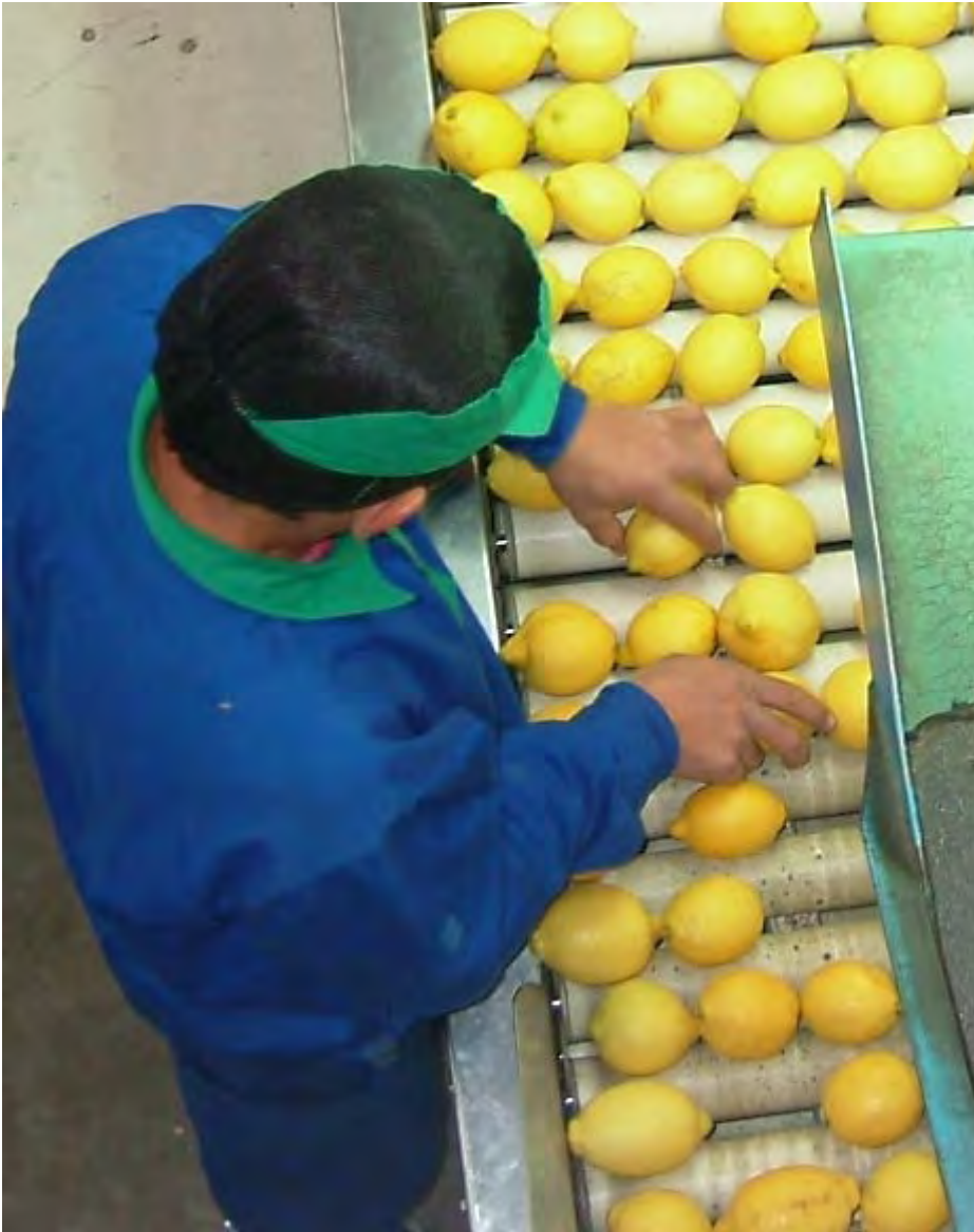
Packing line hand sorting in addition to computer sorting. To comply with SENASA EU requirements. Argenti Pack House, Tucuman, August 7, 2007.
