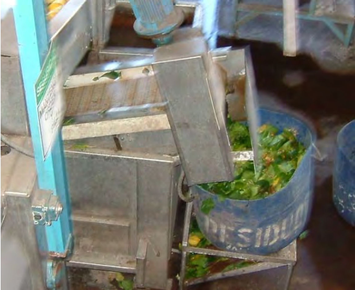
Packing line, automatic removal of leaves and debris from lemons, Argenti Pack House, Tucuman, August 7, 2007.
