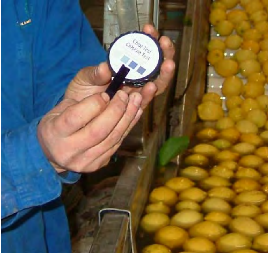
Argenti pack house, monitoring chlorine concentration in water per SENASA EU requirements, August 7, 2007.
