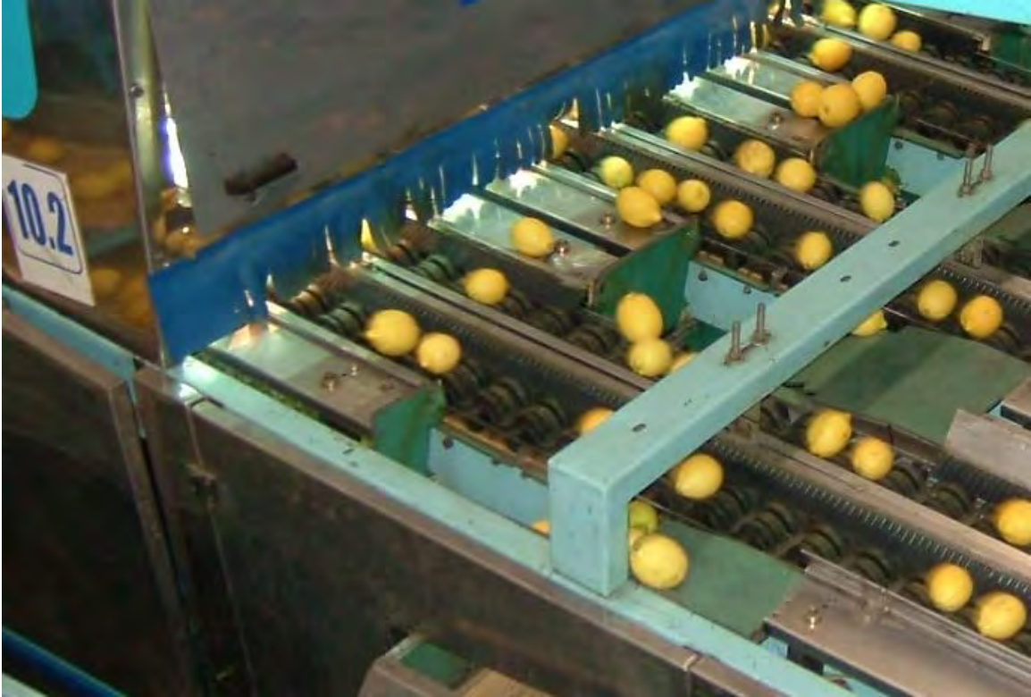
Packing line lemons that have been photographed, analyzed, and selected individually by computer, Argenti Packhouse, Tucuman, August 7, 2007. Rejections seen toppling off the near side of line onto separate conveyor.
