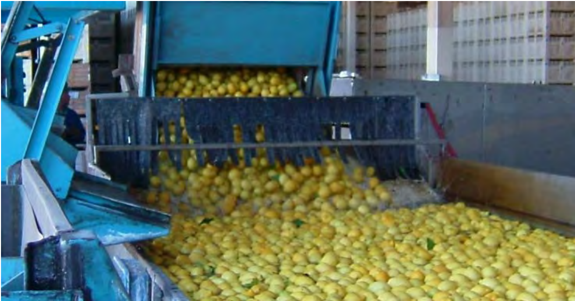
Packing line, dumping bin into 2% sodium hypochlorite per SENASA EU requirement, Argenti Pack House, Tucuman, August 7, 2007.
