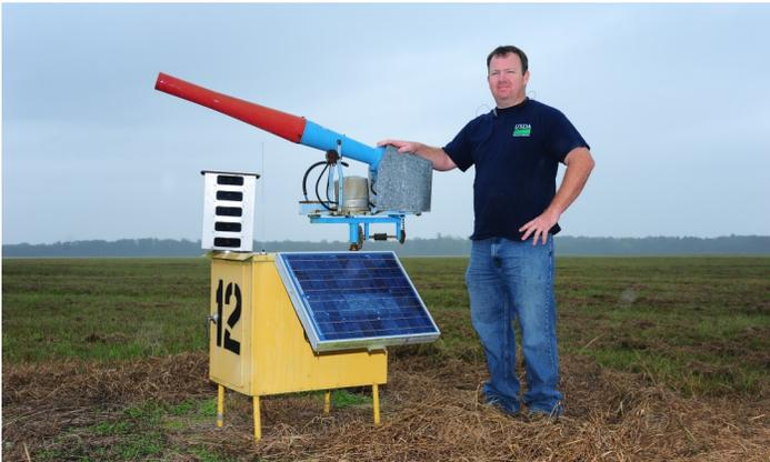
Figure 5. Propane cannons are noise devices used to scare birds and other wildlife.
