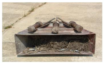
Figure 6. Portable rocket net system.
