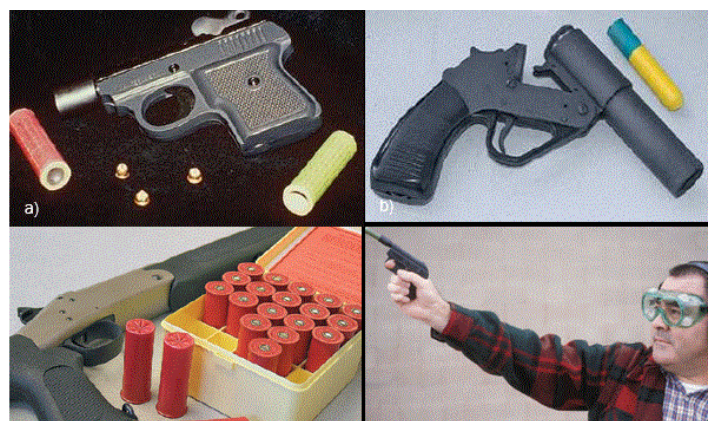
Figure 6. a) 15mm pistol, banger (red) and whistler (yellow) cartridges, (b) 18mm CAPA pistol and cartridge, (c) shotgun used to launch 12-gauge shell crackers, (d) firing a pyrotechnic device.
