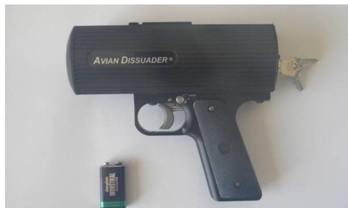
Figure 7. Avian Dissuader laser for dispersing birds.
