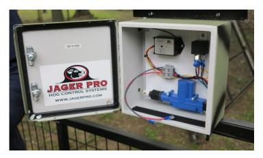
Figure 19. Remote controlled trap trigger.
