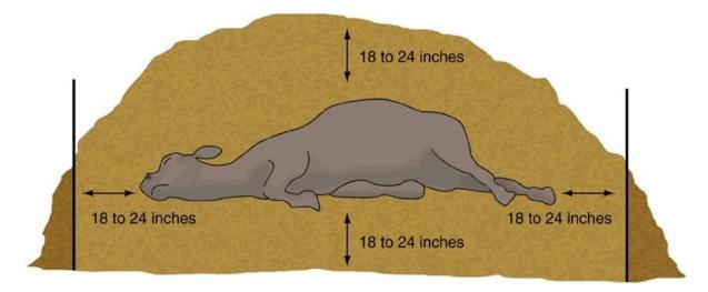
Figure 3. Illustration of carcass location in compost pile.
