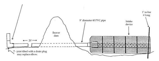
Figures 7. An example of a Clemson pond leveler used to control the water level at a dam.
