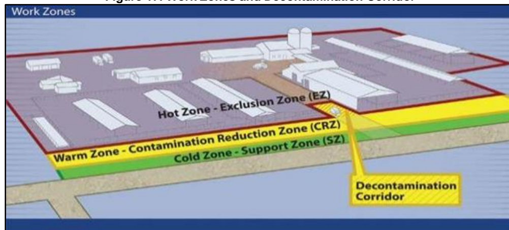
Figure 17. Work Zones and Decontamination Corridor
