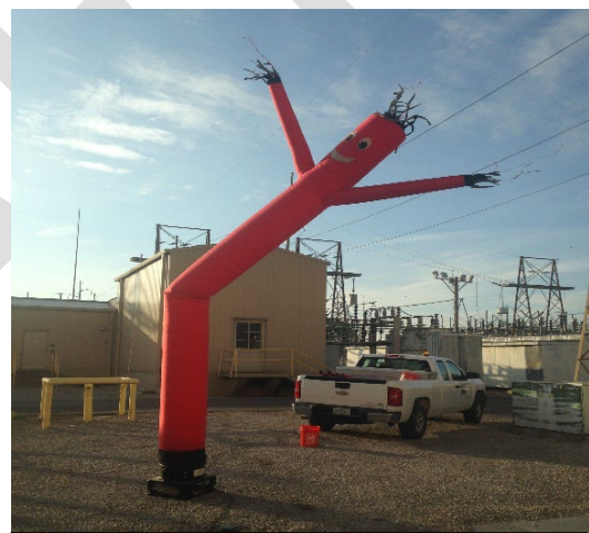
Figure 6. Air dancer installed at a facility to deter flocking birds.
