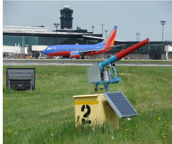
Figure 7. Propane cannon installed on an airport greenbelt to deter birds.
