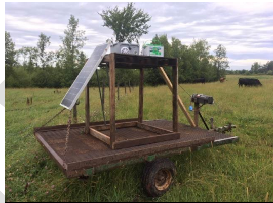
Figure 8. Mobile scare radio electronic deterrent device for wolf damage management.
