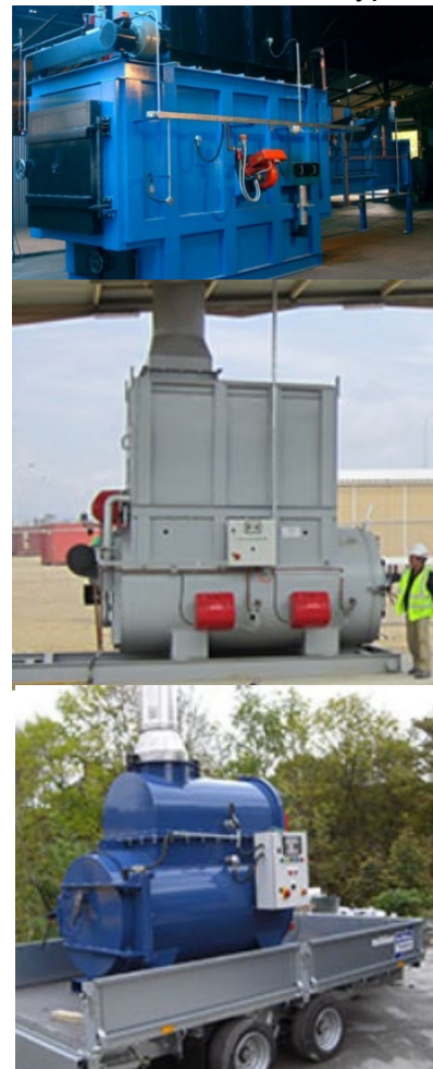
Figure 8. A fixed-facility incinerator, a semi-mobile incinerator on a skid, and a mobile incinerator (picture source matthewsenvironmental.com 2020).
