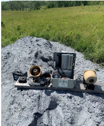
Figure 4. Radio Activated Guard Box; Shown Ineffective at Deterring Radio Collared Wolves. (Sheep Ranch, St. Louis County, MN)
