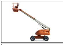
Figure 2. A cherry picker boom which is used to reach nests in high places. *Picture from http://lyexpo.com/.*
