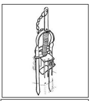
Figure 3. A harpoon -style mole trap, which works best for star-nosed moles. *(Henderson 1994)*
