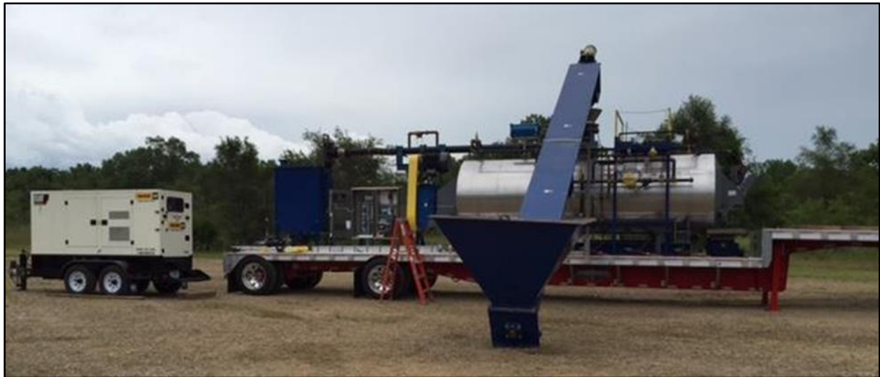
Figure 8. Enviro-Safe Treatment Solutions Mobile Autoclave (Printed with permission from Enviro-safe Treatment Solutions)
