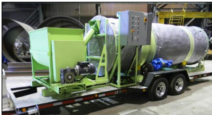
Figure 6. Mobile Rotary Kiln
