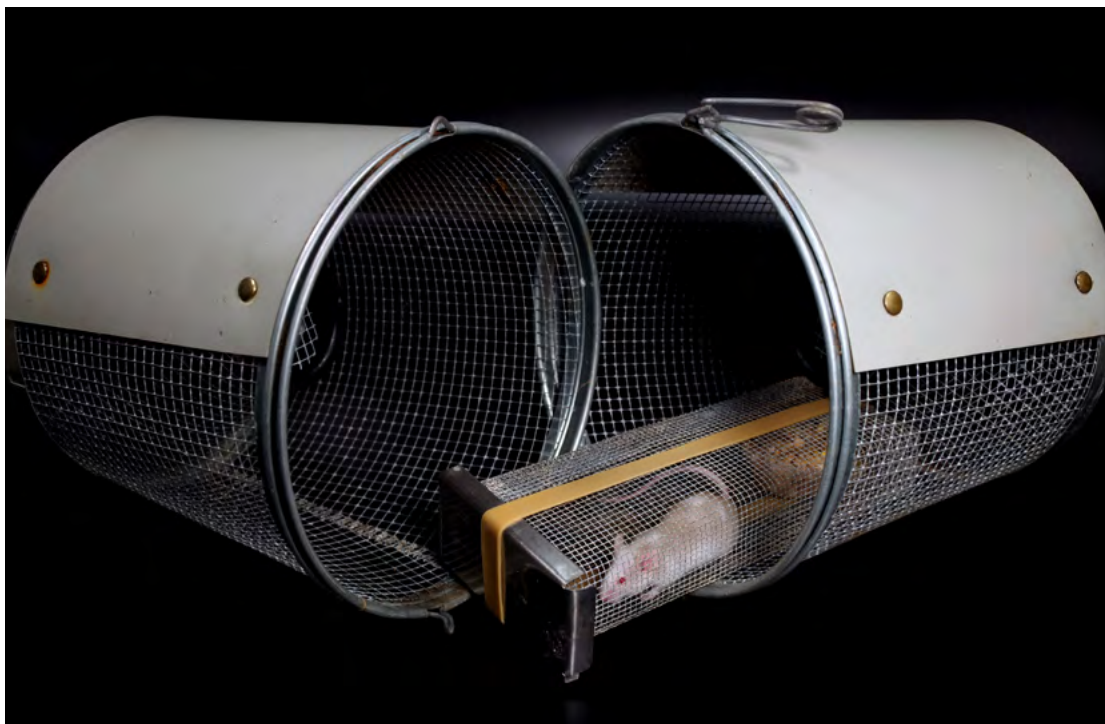
In Guam, traps baited with live mice (mouse-lure traps) are used to remove invasive brown treesnakes.
