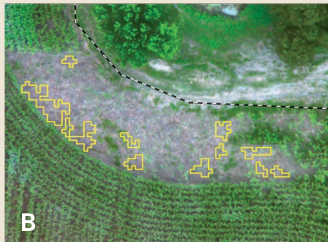
Estimates of feral swine damage to a cornfield using visible and near-infrared information (left) versus only visible information (right) collected from sensors mounted on small, unmanned aircraft systems. Photo by USDA, Wildlife Services
