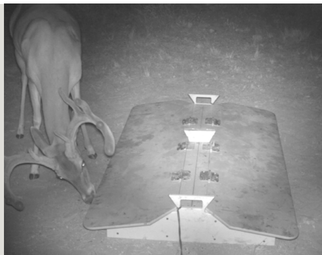
NWRC researchers and Australian partners developed a bait station for feral swine that prevents white-tailed deer and raccoons from accessing the bait.
