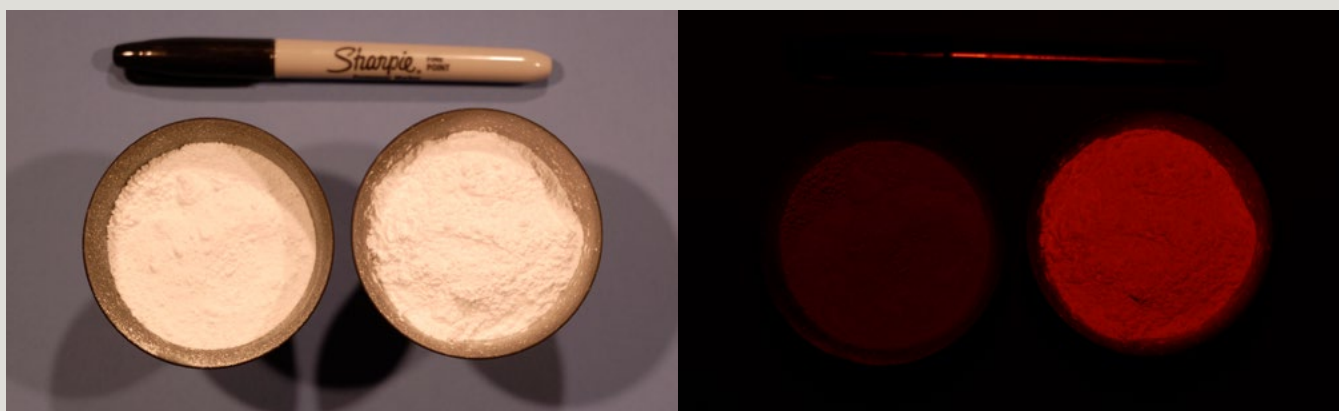
Anthraquinone (AQ) is used as a bird repellent in part due to visual cues related to the compound's absorption of the ultraviolet (UV) spectrum. These pictures show human-visible (left) and ultraviolet images (right) of the UV-absorbent feeding cue and the UV-reflective feeding cue used to test conditioned food avoidance among red-winged blackbirds. Note how the UV-reflective feeding cue is orange in color. USDA solely owns one patent, co-owns one patent, and co-owns three patent applications for AQ technologies with a private company. Photos by USDA, Scott Werner
