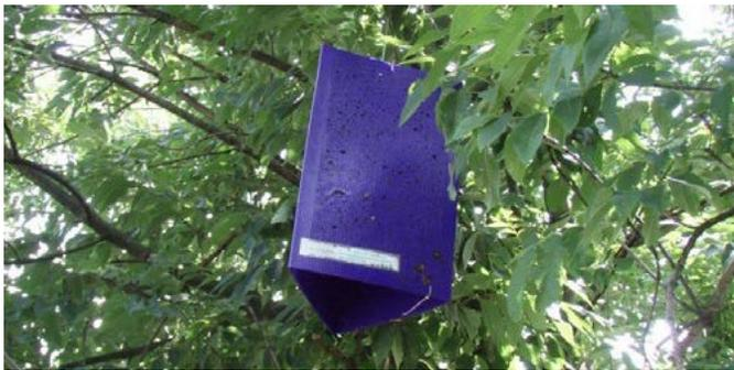
The purple trap is a three-dimensional triangle or prism. It's made out of thin, corrugated purple plastic that has been coated with non-toxic glue on all three exterior sides. The purple traps are about 24 inches long and hang vertically in ash trees. Each trap is baited with a lure on the interior to attract EAB to it.
