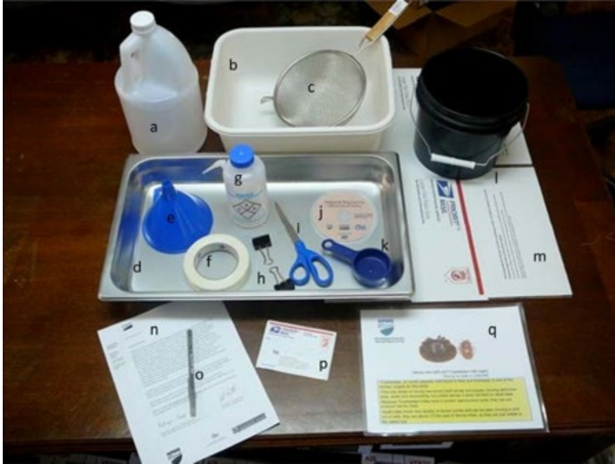
Figure 1: Reusable equipment needed for sampling apiaries. Materials include (a) 1 gallon bottle (to be filled with water), (b) wash tub, (c) strainer, (d) metal pan, (e) funnel, (f) clear binding tape, (g) squeeze bottle (to be filled with water), (h) binder clips, (i) scissors, (j) training video, (k) \frac{1}{4} cup measuring cup, (l) bucket, (m) 3 large Priority Mail flat rate boxes, (n) letters explaining the purpose of this sampling (a copy of this should be given to cooperating beekeepers), (o) pen, (p) 3 preaddressed mailing labels, (q) Tropilaelaps information sheet.
