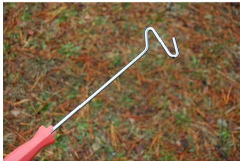
4. The trap can be taken down and serviced by slipping the attachment on the pole through the loop at the top of the hanger, and lifting it off of the tree, and then down to the ground.
