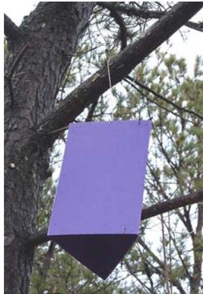
5. In high wind areas, we suggest tying a rope to the bottom loop in the spreader (through the inside of the trap). This rope can be tied to the tree, to help secure the trap.
